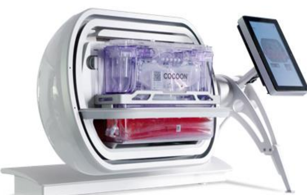
Figure 1. Lonza Cocoon® Platform and Cocoon® Cassette. Functionally closed, highly customizable and scalable integrated cell manufacturing platform. Whether it is a centralized or decentralized cell manufacturing model, the Cocoon® Platform approach reduces costs and supports manufacture of robust cell therapy products.
